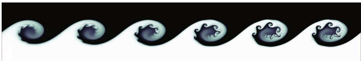
Figure 8.6: Temporal development of the Kelvin-Helmholtz secondary instability in a sheared fluid constituted of two layers, with the black fluid being three times denser than the white fluid. After Fontane et al. , Phys. Fluids 20 , 091109 (2008).
