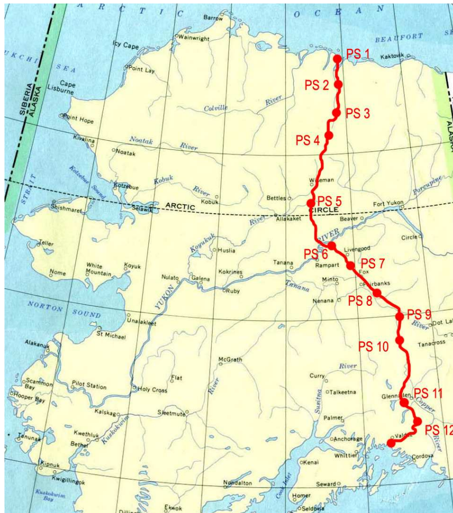
Figure 1.2: Map of the Trans-Alaska Pipeline System shown by the red line, going from Prudhoe Bay (North) to Valdez (South). The red dots labelled PS indicate pump stations (note: PS 11 was never built). More details can be found on http://www.alaska-pipe.com/ and http://en.wikipedia.org/wiki/Trans-Alaska_Pipeline_System .
