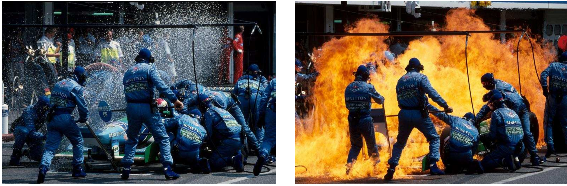
Figure 1.4: Formula 1 pit stop of Jos Verstappen (Benetton). The fuelman released the hose too early and fuel spilt around the car (left). A fraction of a second later, with the engine on, a fire was set (right).
