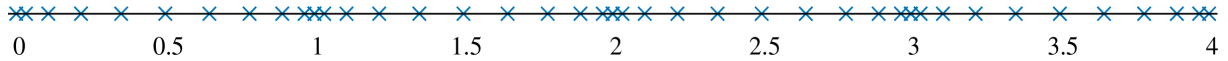
Figure 8: Representation of an Gauss–Lobatto–Legendre element discretization of the interval [0, 4] using 4 identical elements of 11 points each.
