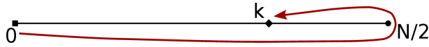
Figure 5: Graphical representation of the frequency folding phenomenon. In order of ascending wavenumber, modes project onto themselves until the Nyquist frequency, N/2 , then spuriously down until wavenumber 0 before going back up again in a periodic process. The idea behind dealiasing via Fourier filtering is to filter out modes with wavenumber larger than k in such a way that when the non-linearity is applied to a mode of wavenumber k , frequency folding occurs but does not reach back to k , as shown by the dark red arrow.
